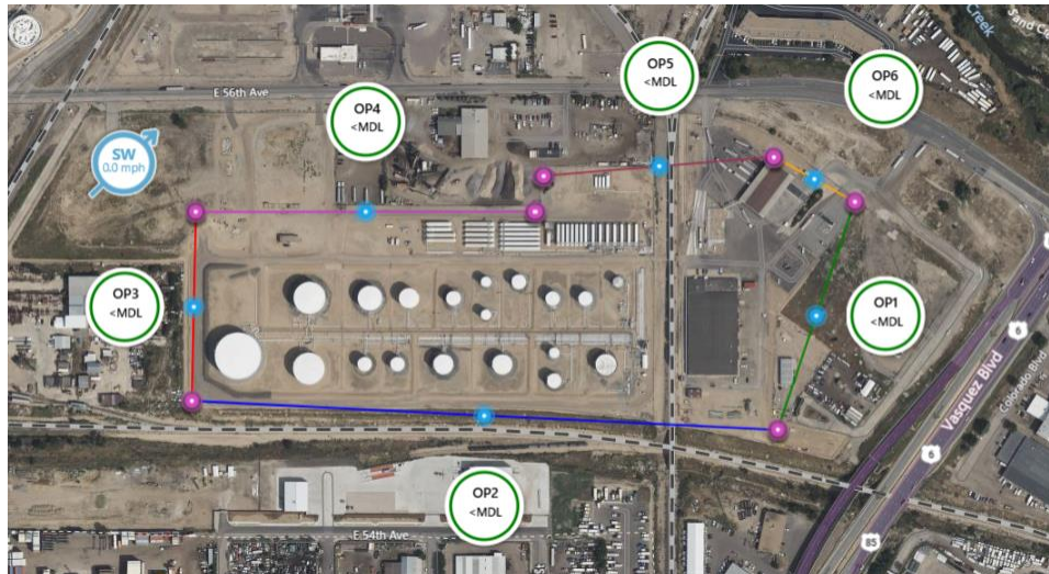
Figure 1: Approximate Layout of the Open-Path Analyzers, Retroreflector Locations, and Meteorological Station
